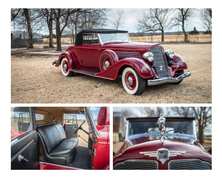
This particular 1934 Buick 66C, was one of 235 series 60s manufactured with the attractive Convertible Coupe/Rumble Seat bodywork. Of the 235 manufactured, this is believed to be one of the 10 earmarked for export. It is powered by the overhead valve 278ci straight eight, and fitted with a synchronized 3 speed transmission.
