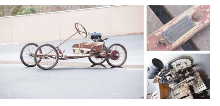
The Red Bug was conceived as a simple low cost automobile. Powered either by Smith Motor Wheels or by electric propulsion. Their lightweight and simplicity made them quite popular. Notable customers even include "Le Patron" Ettore Bugatti.
