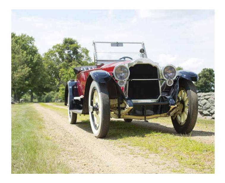
An Oklahoma oilman ordered this custom Packard 3-35 Ormonde in 1918. Standing six foot five the purchaser had Rubay make special accommodation for his height. In order to accommodate the tall driver the steering column was lengthened six inches and lowered to a dramatic rake. The doors were lengthened and the seat set unusually far back from the pedals for a car of the day. All the custom requests delayed the production of the car and he is said to not have received it until 1920.
