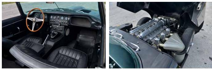
including its matching-numbers 4.2L inline six cylinder with triple SU carberators, and 4-speed manual gearbox.
