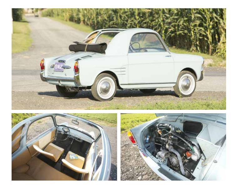
With their peppy, air cooled, rear mounted 2 cylinder engines, 4-speed manual gearboxes, 4-wheel independent suspension, and 4-wheel hydraulic drum brakes, Autobianchi Bianchina's are excellent examples of some of the world's finest micro cars.
