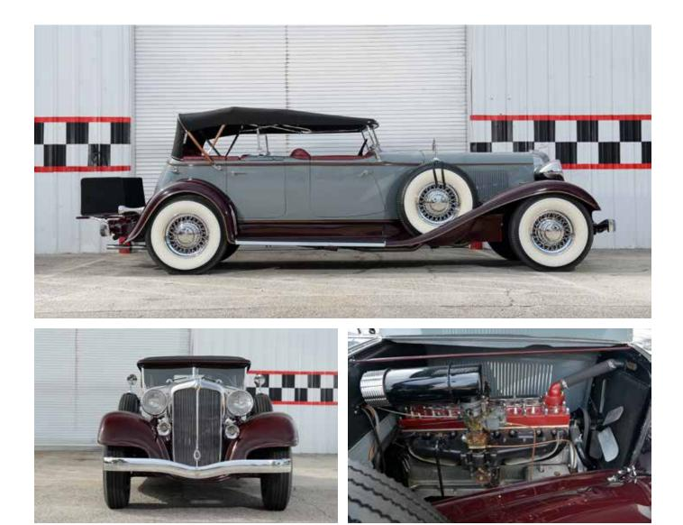
shell was overtly Cord-like, and as with the L-29, the Imperial windshield was set far back on the chassis, permitting a very long hood/cowl line and gracefully sweeping front fenders. With its 145 inch wheelbase chassis being even longer than the L-29, the Imperial's proportions were all the more breath-taking.
