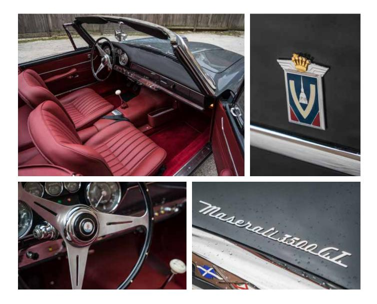
version were the work of Carrozzeria Vignale. Introduced in 1959, Vignale's Maserati 3500GT Spyder was the creation of Giovanni Michelotti, at that time the company's star designer. Built on a slightly shorter wheelbase - 250cm as opposed to 260cm - than the coupé and constructed of steel panels rather than the closed car's aluminum, the spyder lasted in production until 1964, by which time only 245 cars had been made.
